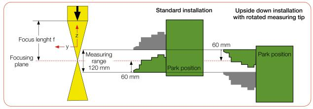
Fig. 7.4: Position of the device relative to the laser beam
