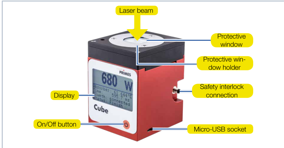
Fig. 5.1: System description of the Cube M
