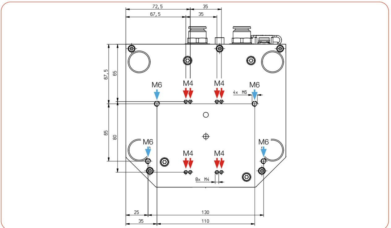
Fig. 6.4: Mounting threads M4 and M6 in the bottom of the housing of the CPM+ F-10 (dimensions in mm)
