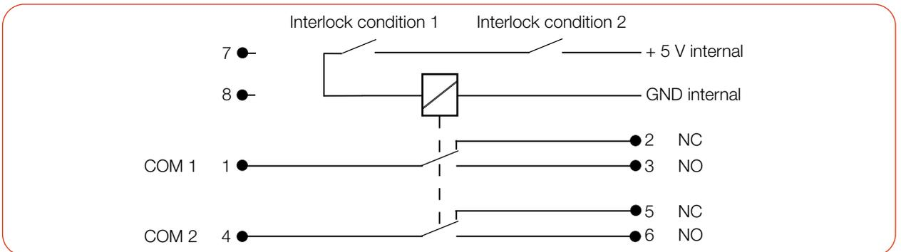
Fig. 7.7: Circuit diagram: Monitored operating conditions (Interlock conditions)
