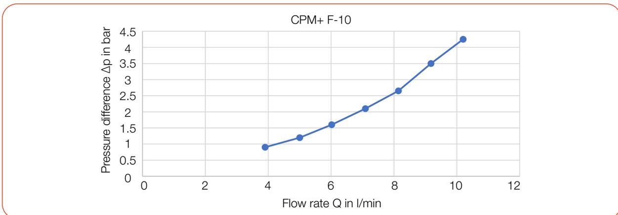
Fig. 7.10: Pressure loss diagram CPM+ F-10
