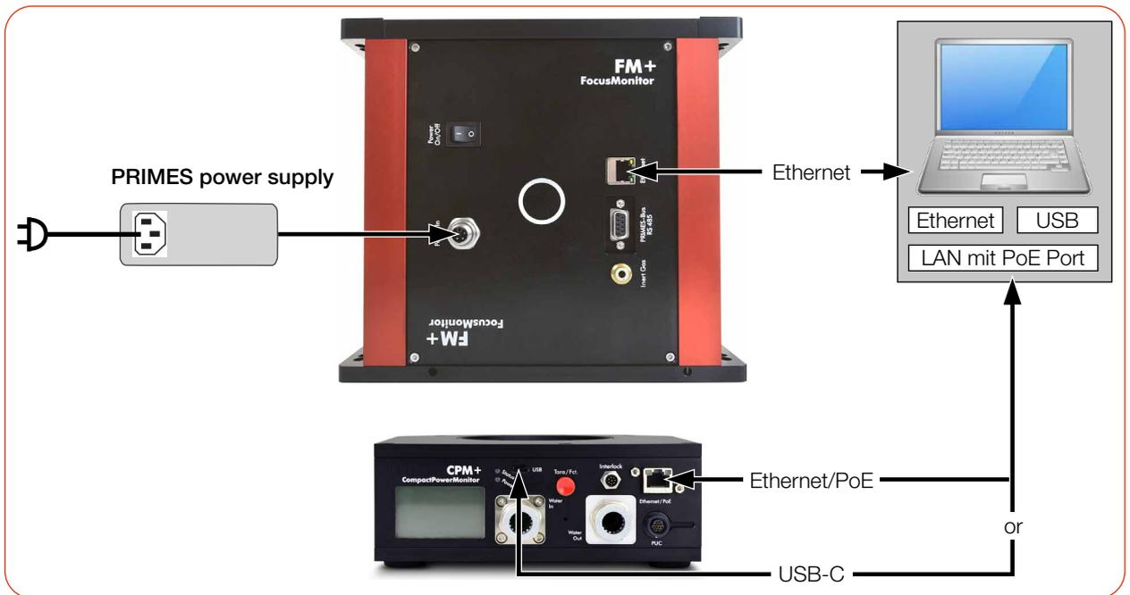
Fig. D.1: Connecting the FocusMonitor FM+ to the CPM+ (using the CPM+ F-10 as example)
