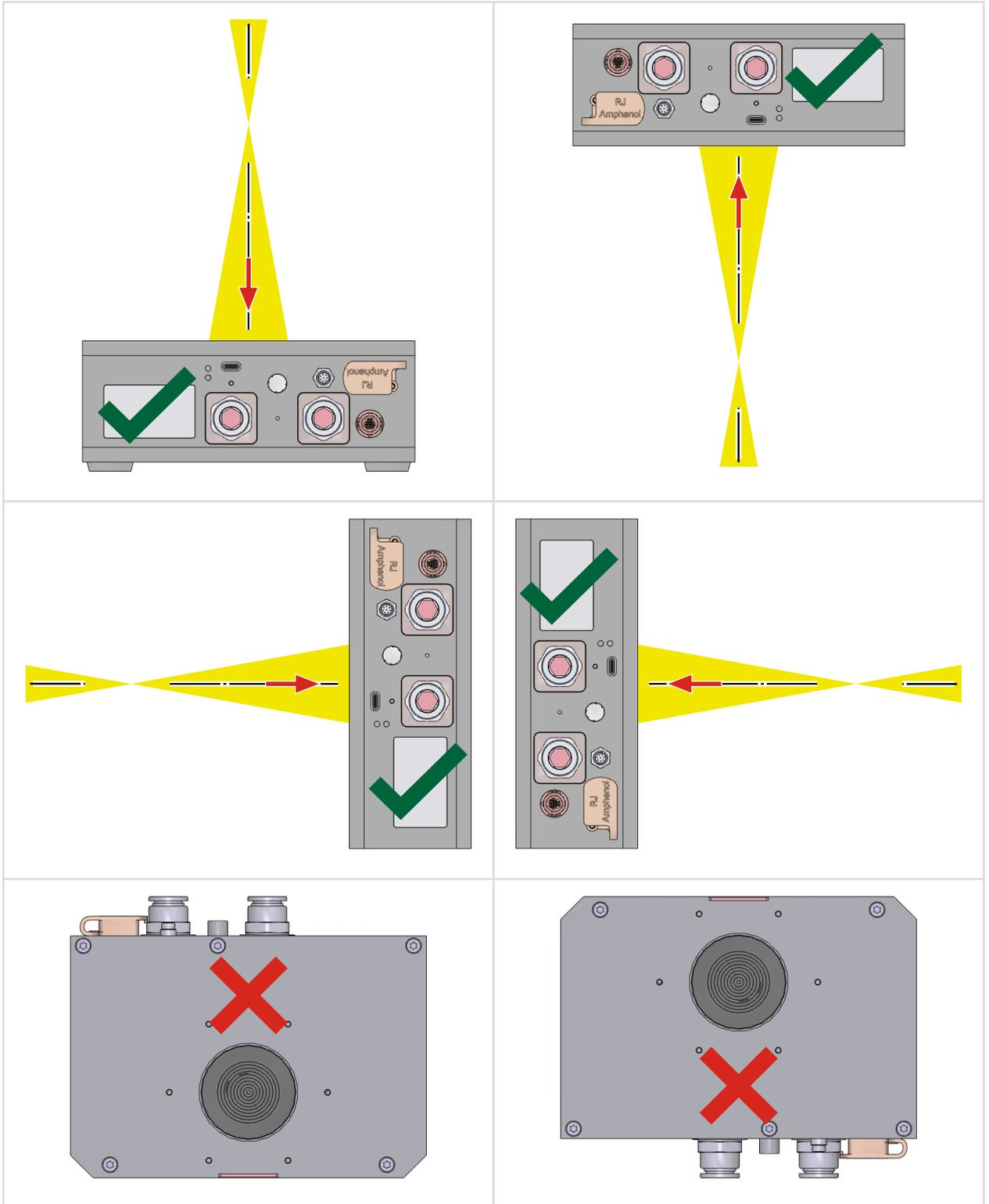
Fig. 6.1: Mounting positions of the CPM+ F-1
