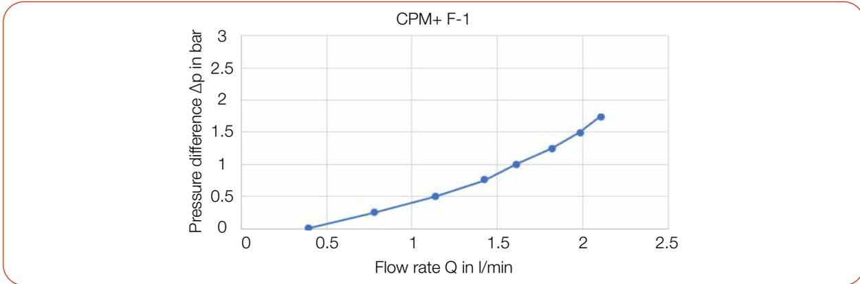
Fig. 7.9: Pressure loss diagram CPM+ F-1
