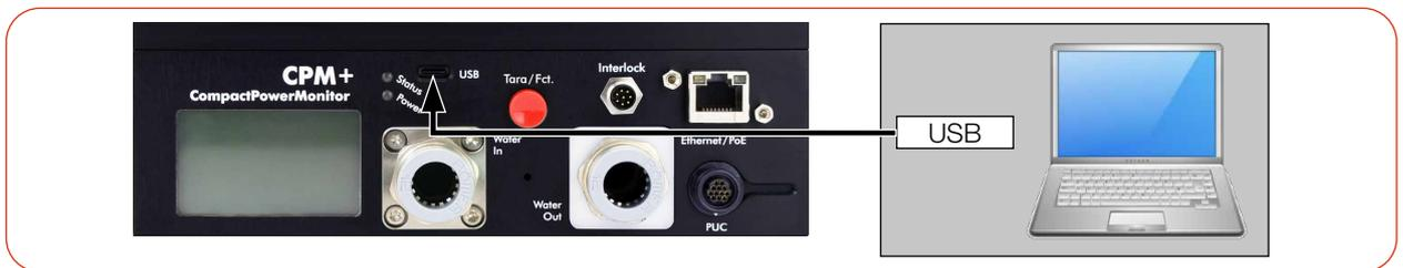
Fig. 7.3: Power supply via USB, data transfer via USB
