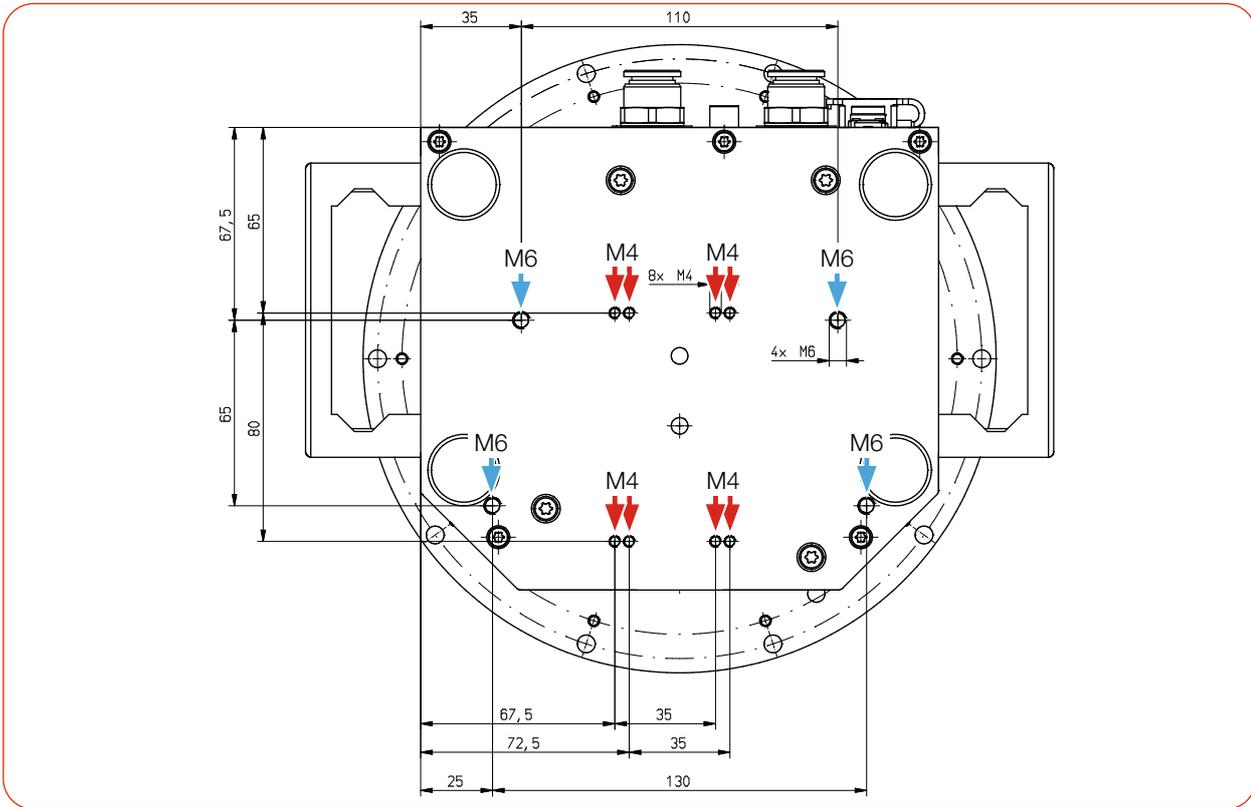
Fig. 6.5: Mounting threads M4 and M6 in the bottom of the housing of the CPM+ F-30 (dimensions in mm)
