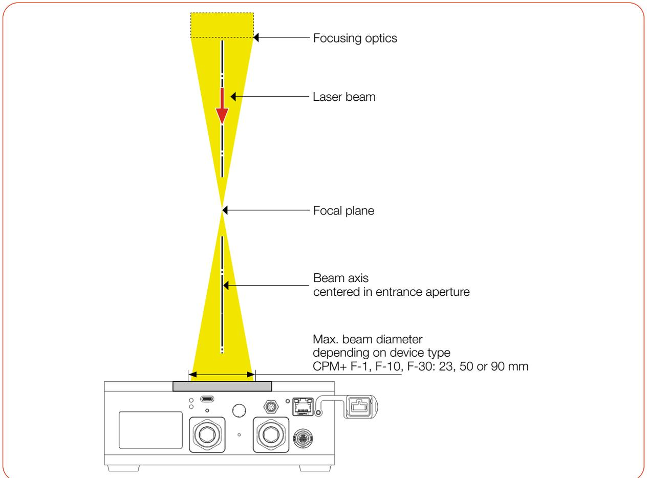
Fig. 6.2: Alignment of the CPM+ to the laser beam using the CPM+ F-10 as example (schematic)
