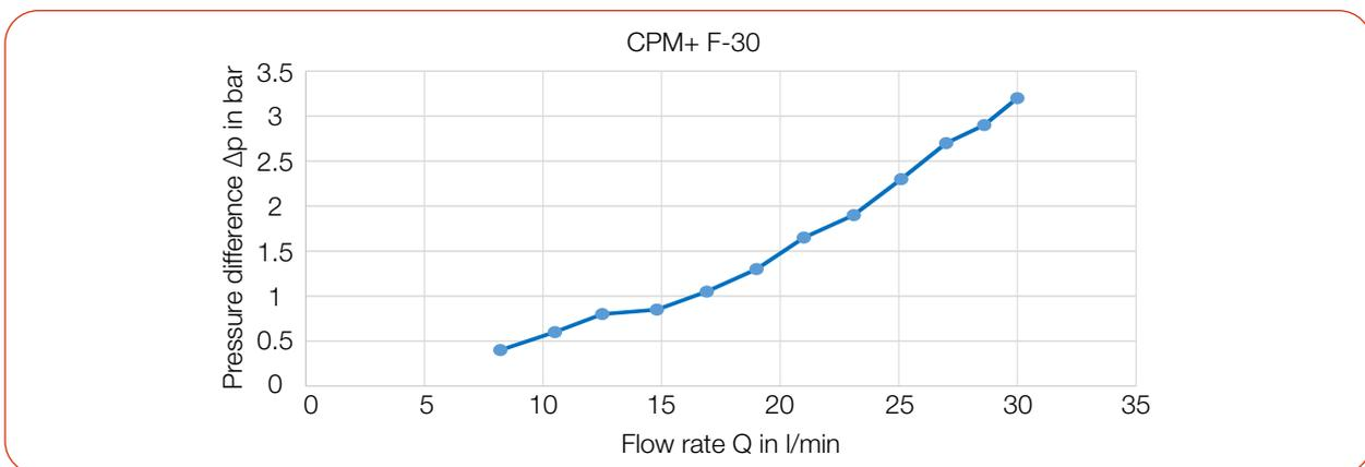
Fig. 7.11: Pressure loss diagram CPM+ F-30
