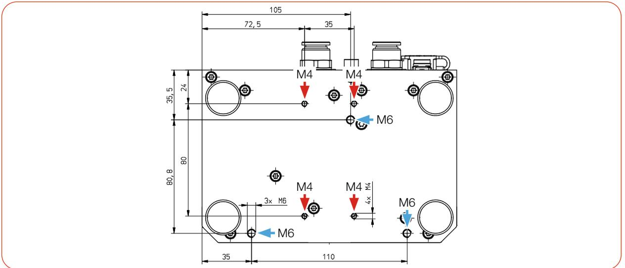
Fig. 6.3: Mounting threads M4 and M6 in the bottom of the housing of the CPM+ F-1 (dimensions in mm)
