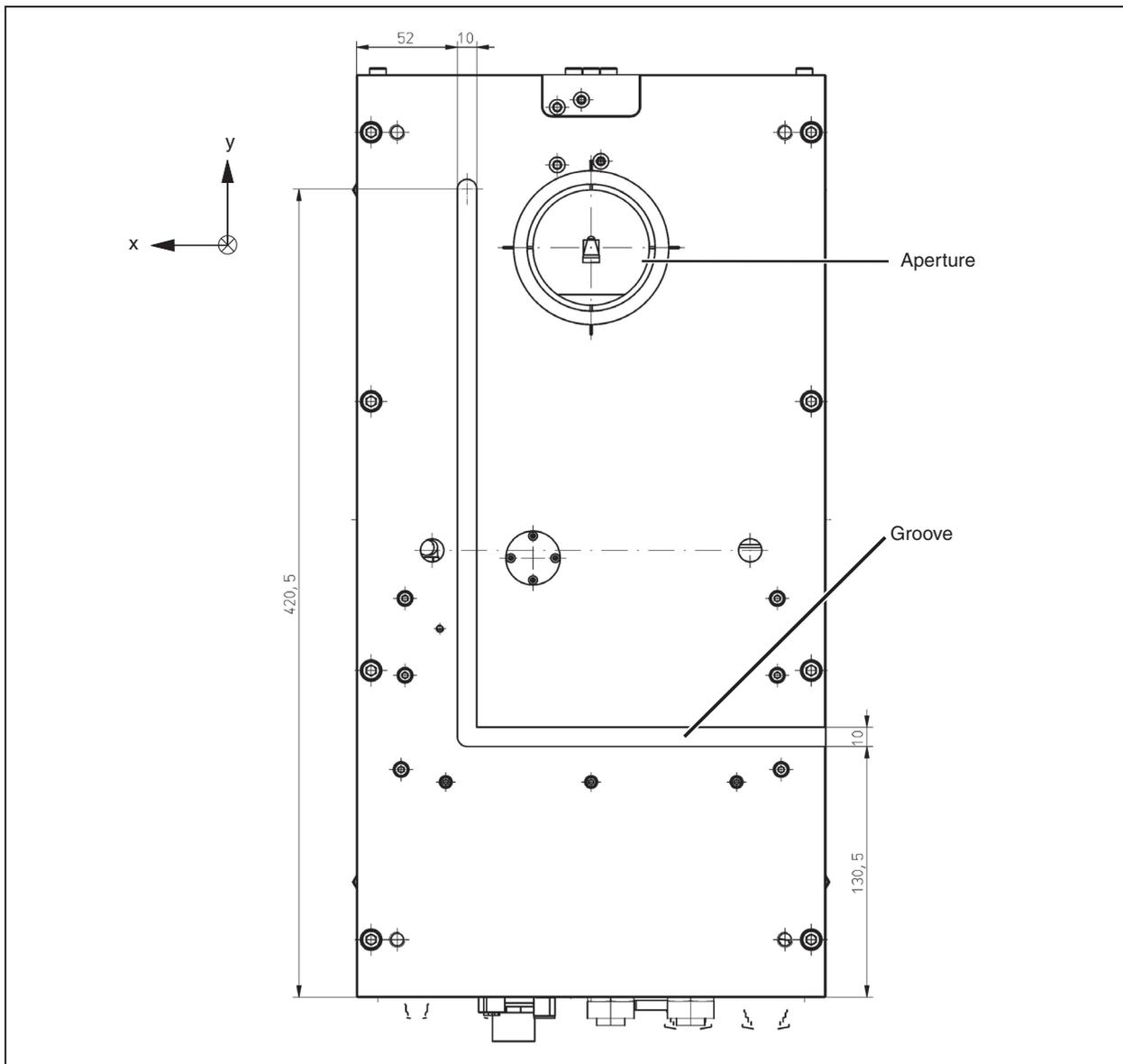
Fig. 7.1: Groove dimensions, view from above
