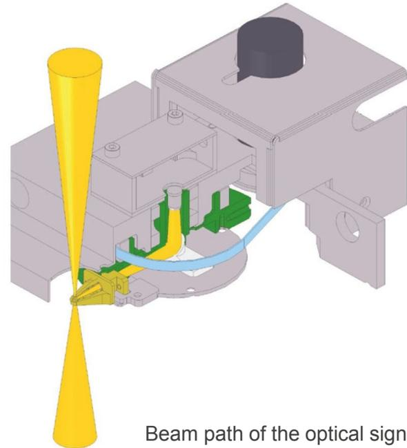
Beam path of the optical signal
