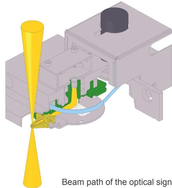
Beam path of the optical signal
