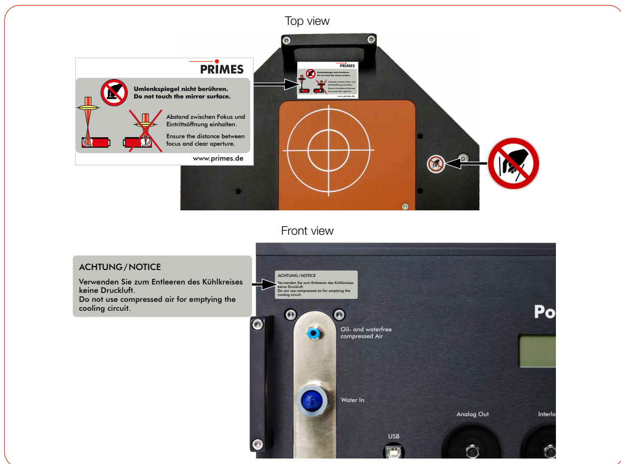
Fig. 4.3: Product safety label “Do not reach inside” and warning labels (using the PM 100 as example)
