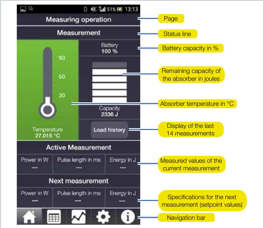
Fig. 3.3: Measuring operation
