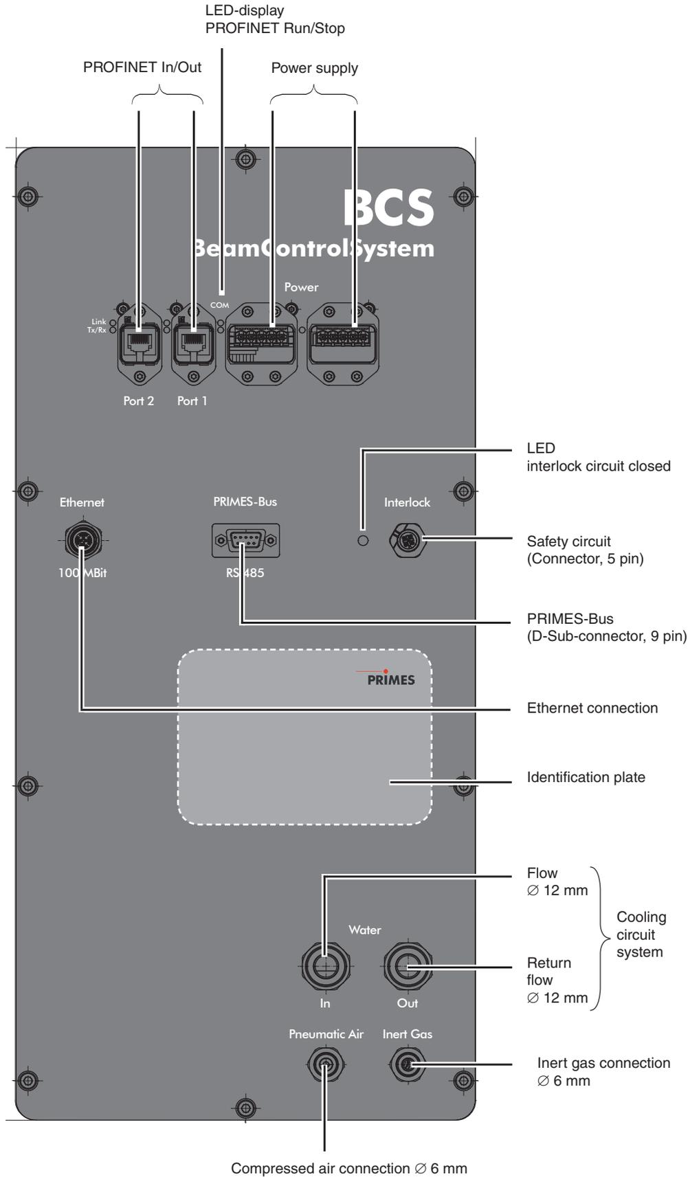
Fig. 6.1: Overview of connections
