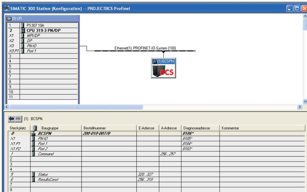
Fig. 10.1: Integration of the GSDML – file under step 7
