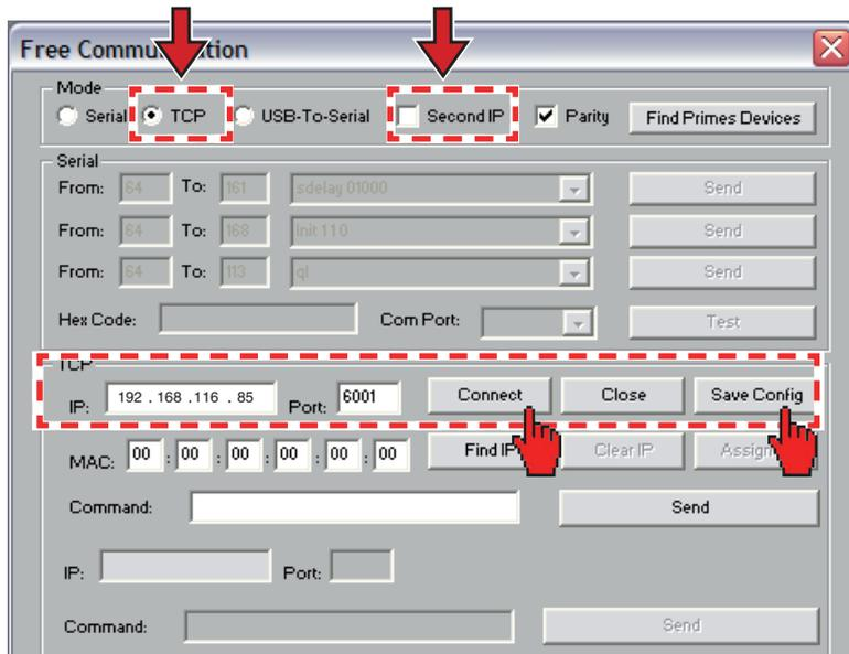
Fig. 11.1: Establishing a connection in the menu *Free Communication*
