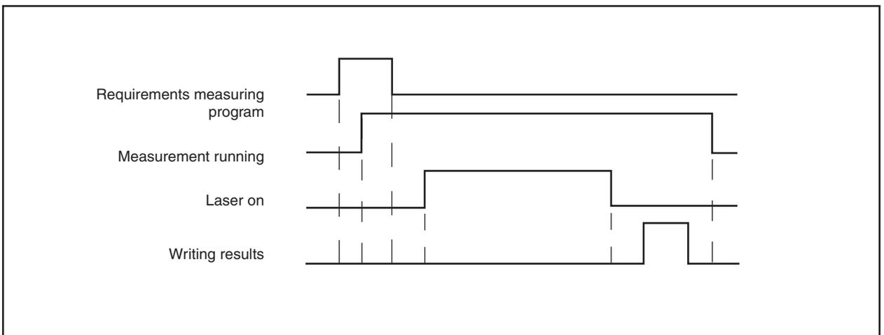
Fig. 12.1: Simplified timing diagram of the measuring procedure
