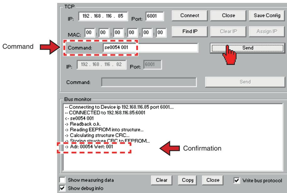
After a newstart of the device with the network connection now the router/server will be asked for an IP-address. Now the Server will activate a new address which needs to be requested via your router/server. The function FINDIP over the MAC address (image no.4) is not working than.
