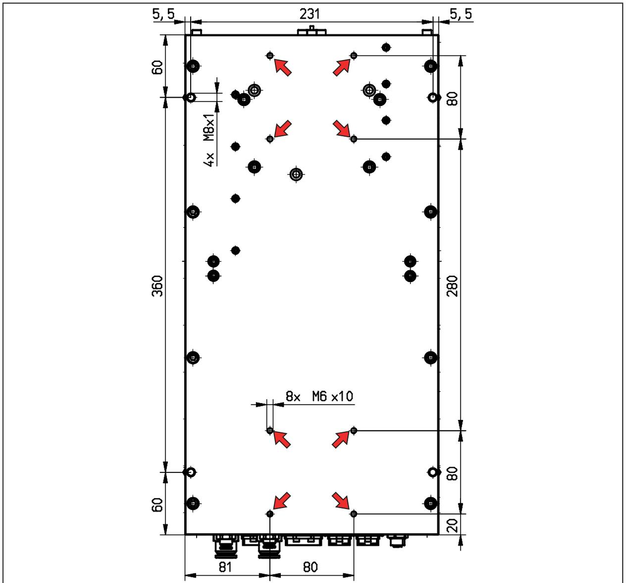
Fig. 7.3: Fixing holes, view from bottom
