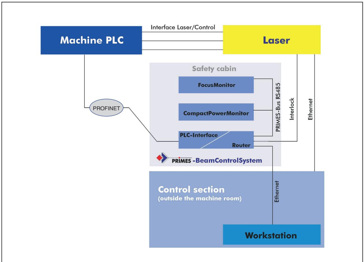
Fig. 5.2: Principle of the electrical integration of the BCS
