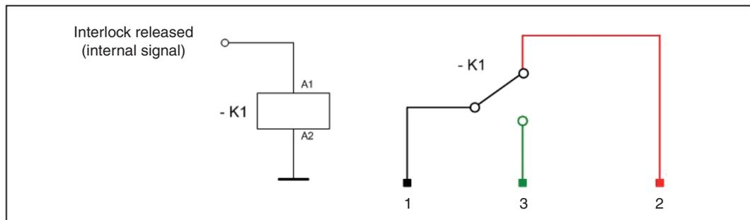
Fig. 9.1: Circuit diagram of the safety circuit
