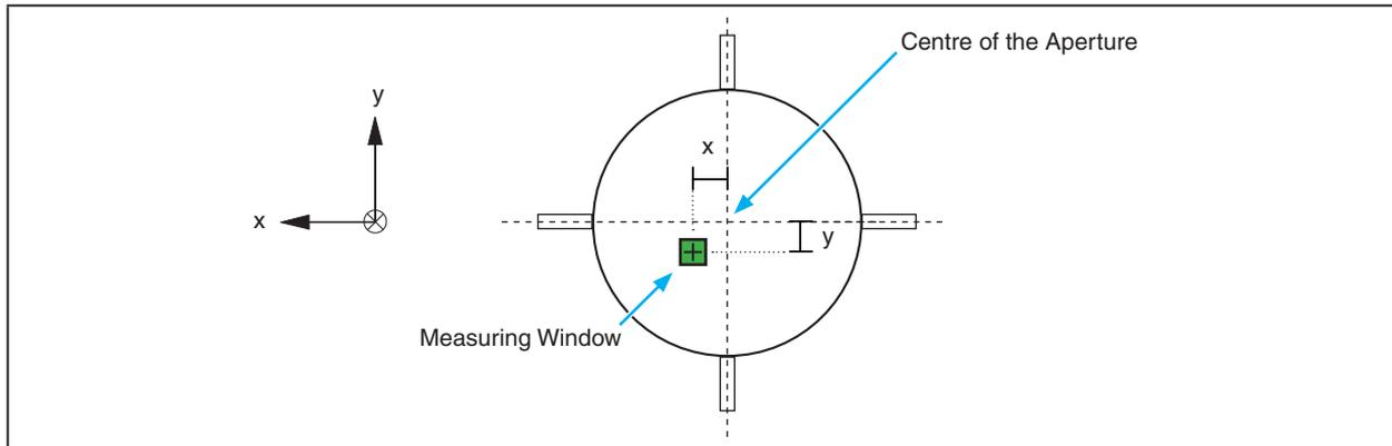
Fig. 7.2: Distances centre of the aperture – centre of the measuring window
