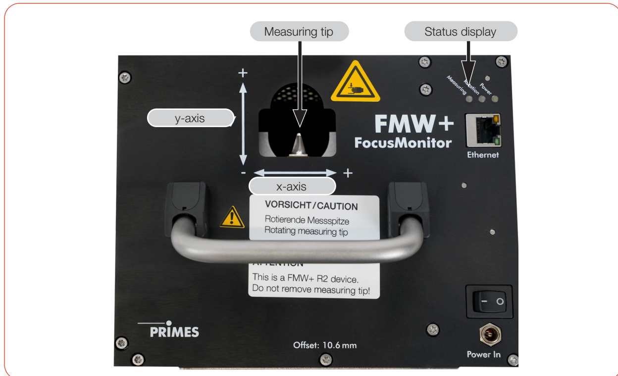
Fig. 4.1: Main components FMW+ R2
