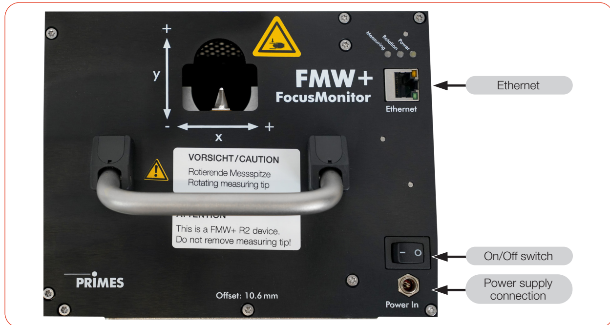
Fig. 8.1: FMW+ R2 connections
