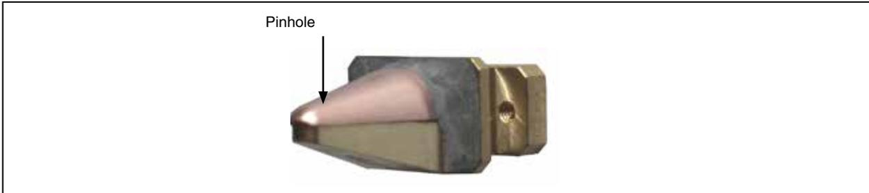
Fig. 15.4: Opening aperture (pin hole) in the measurement tip
