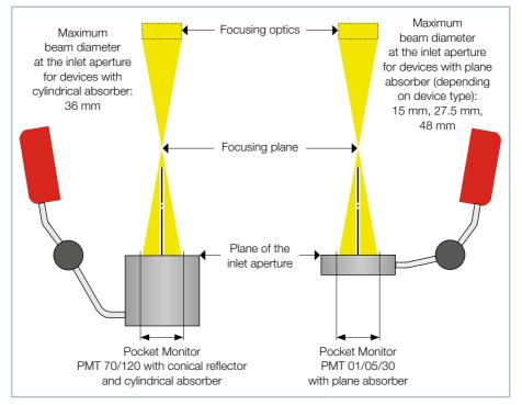
Fig. 9.1: Alignment to the laser beam
