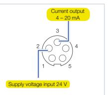
Pin diagram socket (top view, plug-in side)
